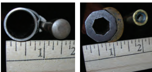
Comparing the bore of a musket (LEFT) and a rifle (RIGHT).
